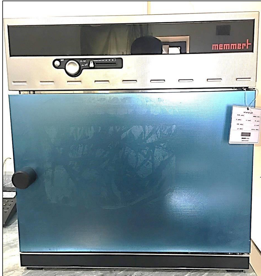
Figure (2.12): Memmert heating and drying oven.
