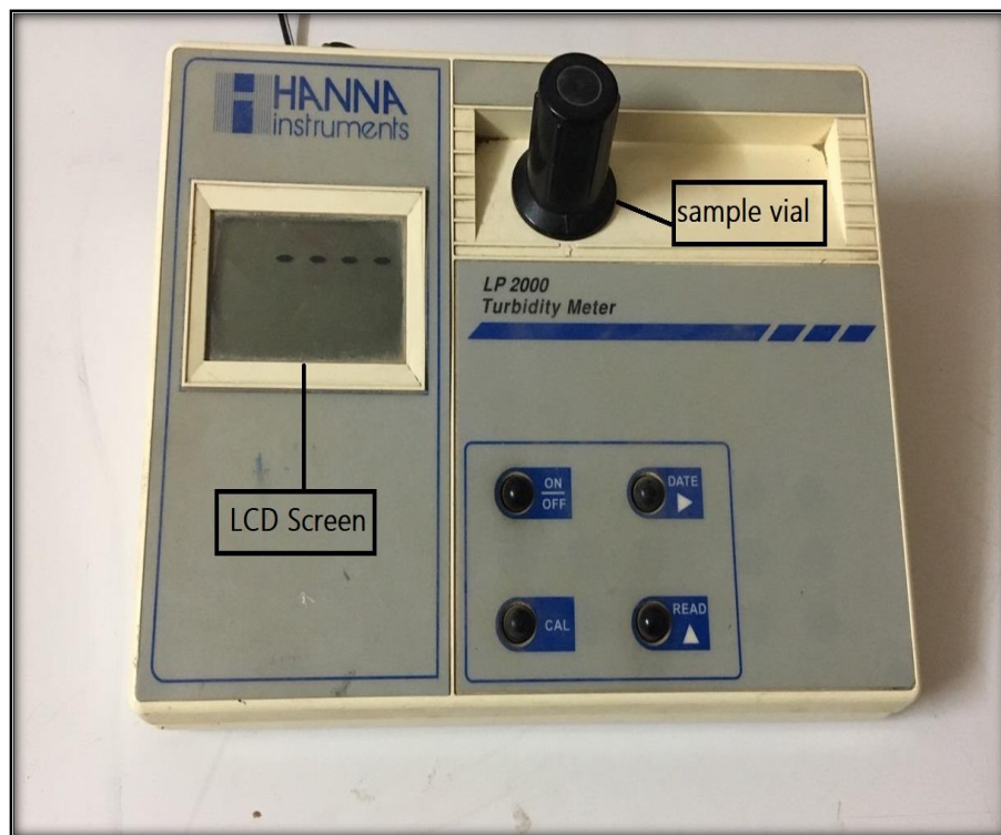
Figure (2.9): LP 2000 microprocessor-based bench turbidity meter.
