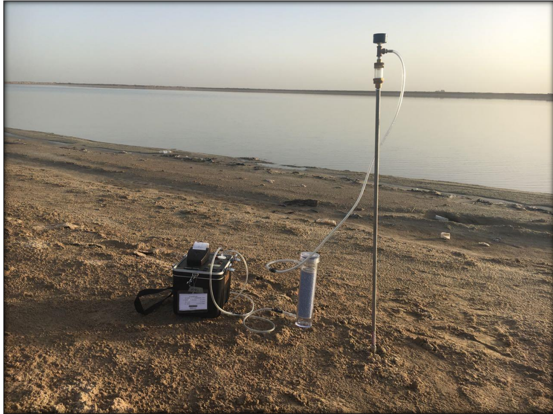
Figure (2.20): Radon soil-gas in situ measurements.
