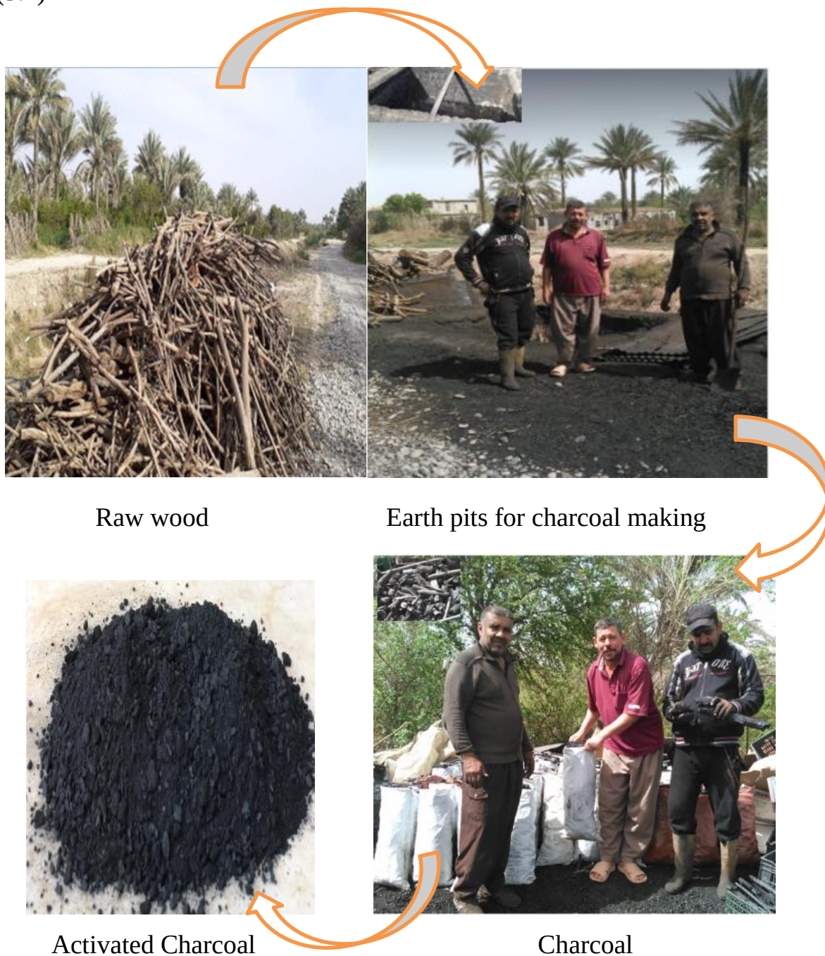
Fig 3.1 The steps of preparation charcoal and activated charcoal in Sinsil Al-Tayeha village - Diyala – Iraq
