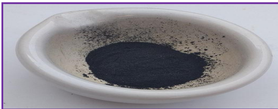
Figure 2.11. Preparation of the \gamma - \text{Al}_2\text{O}_3/\text{AC} nanocomposites produced from \text{Al}_2(\text{SO}_4)_3 \cdot 16\text{H}_2\text{O} and activated charcoal
