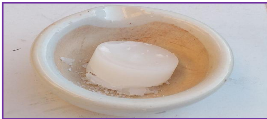
Figure 2.9. Preparation of \gamma - \text{Al}_2\text{O}_3 /paraffine nanocomposite produced from \text{AlCl}_3 \cdot 6\text{H}_2\text{O} and paraffin
