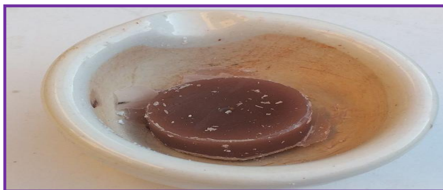
Figure 2.7. Preparation of the \alpha - \text{Fe}_2\text{O}_3 / paraffin nanocomposite from \text{FeCl}_2 \cdot 2\text{H}_2\text{O} with paraffin
