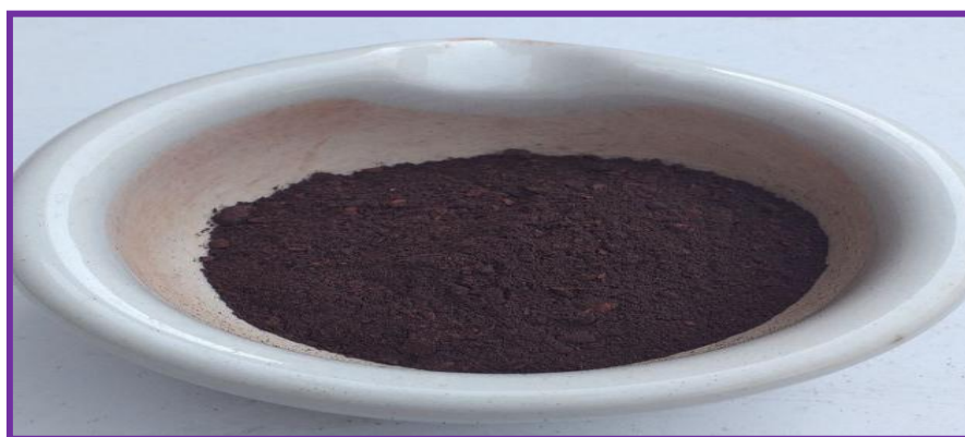
Figure 2.4. Preparation of \alpha - \text{Fe}_2\text{O}_3 nanoparticles from aqueous \text{FeCl}_2 \cdot 2\text{H}_2\text{O} salt
