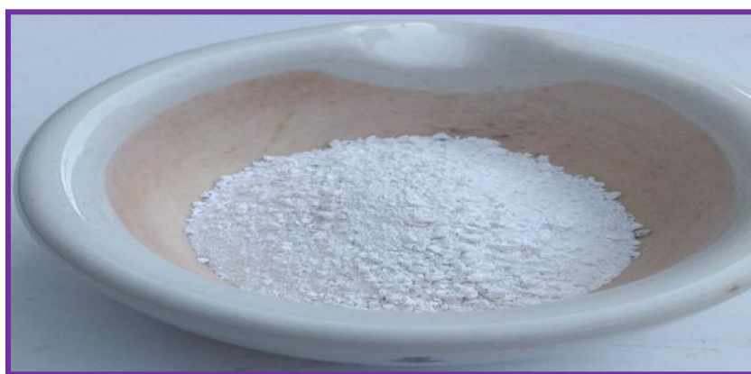
Figure 2.2. Preparation of \gamma - \text{Al}_2\text{O}_3 nanoparticles from aqueous \text{AlCl}_3 \cdot 6\text{H}_2\text{O}
