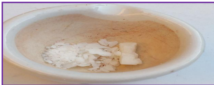
Figure 2.8. Preparation of the \gamma - \text{Al}_2\text{O}_3 /paraffine nanocomposite produced from \text{Al}_2(\text{SO}_4)_3 \cdot 16\text{H}_2\text{O} and paraffin
