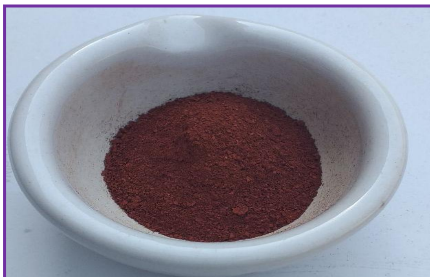
Figure 2.5. Preparation of \alpha -Fe 2 O 3 nanoparticles from aqueous FeSO 4 ·7H 2 O
