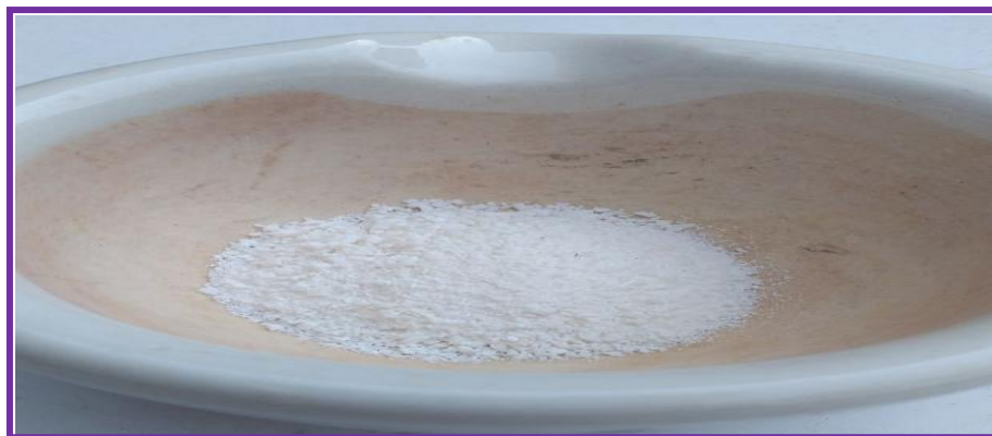
Figure 2.3. Preparation of \gamma - \text{Al}_2\text{O}_3 nanoparticles from aqueous \text{Al}_2(\text{SO}_4)_3 \cdot 16\text{H}_2\text{O}
